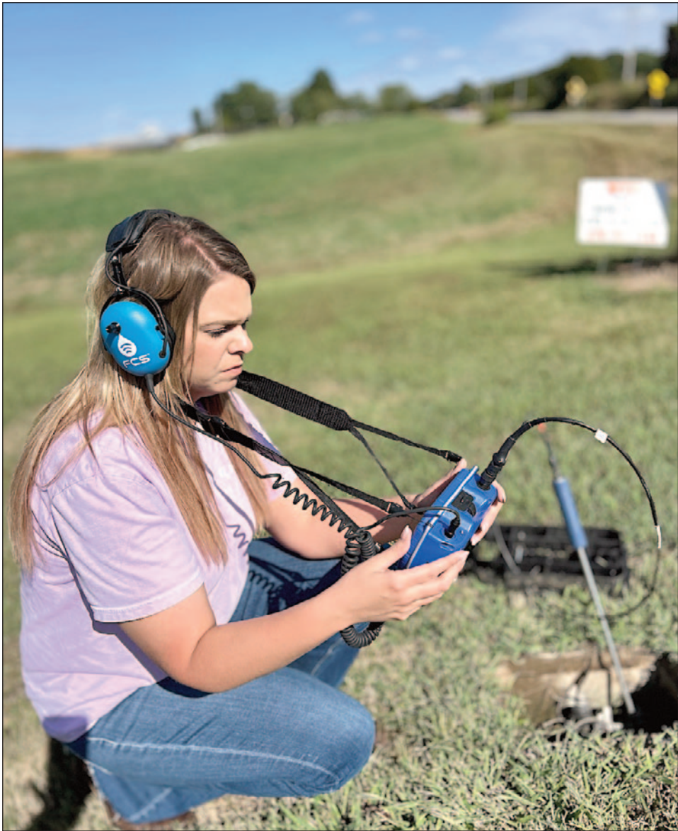
Crittenden-Livingston Water District Superintendent Abbie Adamson is trying to dial in on costly leaks with a listening device that helps find underground problems.
